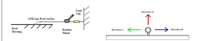
The ANKAme roof anchor has been designed and tested to suite the following roof sheet profiles and concrete;
